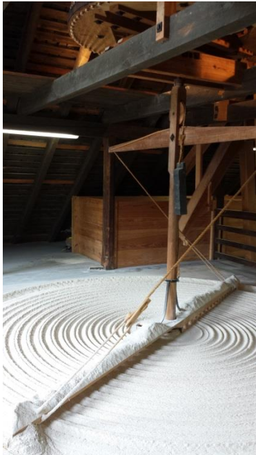
The Hopperboy in action at the George Washington Gristmill. Photo credit: Carol Joyce.
