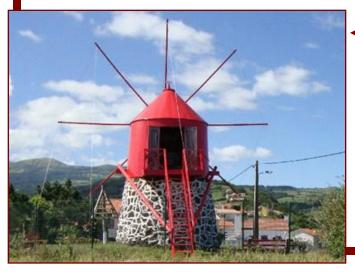
On the islands of Faial and Pico, mills have a truncated cone-shaped stone base with a rotating wooden tower and central staircase that acts as a stabilizing "tail." There is a central mast projecting outward to which 8 poles are wired so as to support triangular sails.
